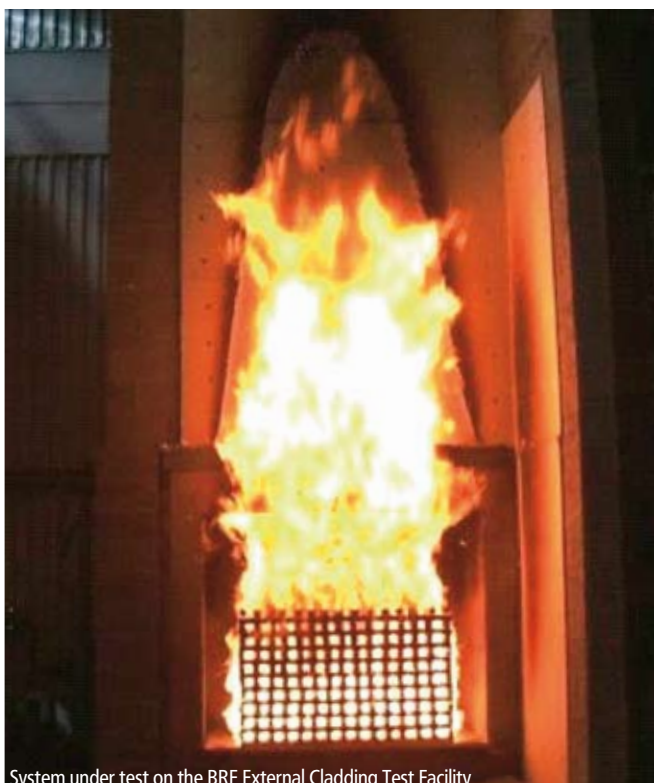
System under test on the BRE External Cladding Test Facility
