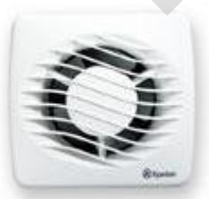
An extractor fan – can be manually controlled, switch on with the lighting circuit, have time delay and sometimes humidity sensors.
