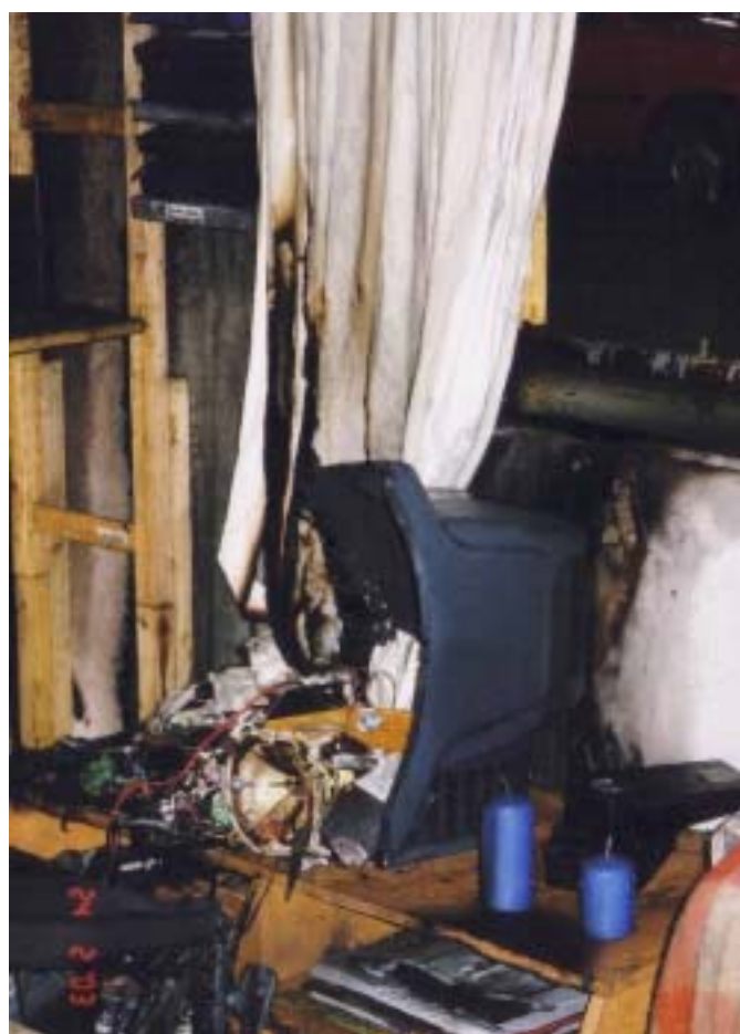
Figure 5B.7 Sprinklered (sprinkler B), open lounge door: Test 5
