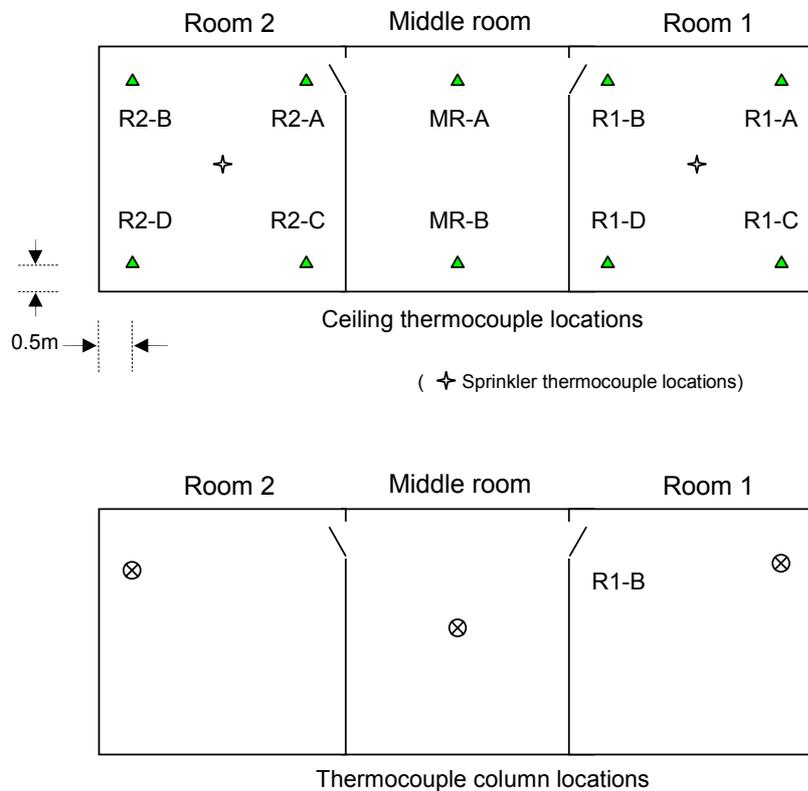
**Figure 5.10 Thermocouple locations**
