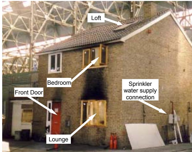
**Figure 5.1** The experimental facility
