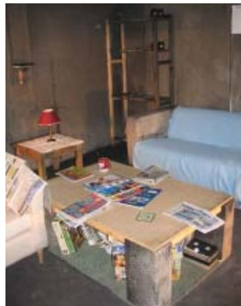
Figure 5.13 Fuel arrangement for table fire (in room 1)
