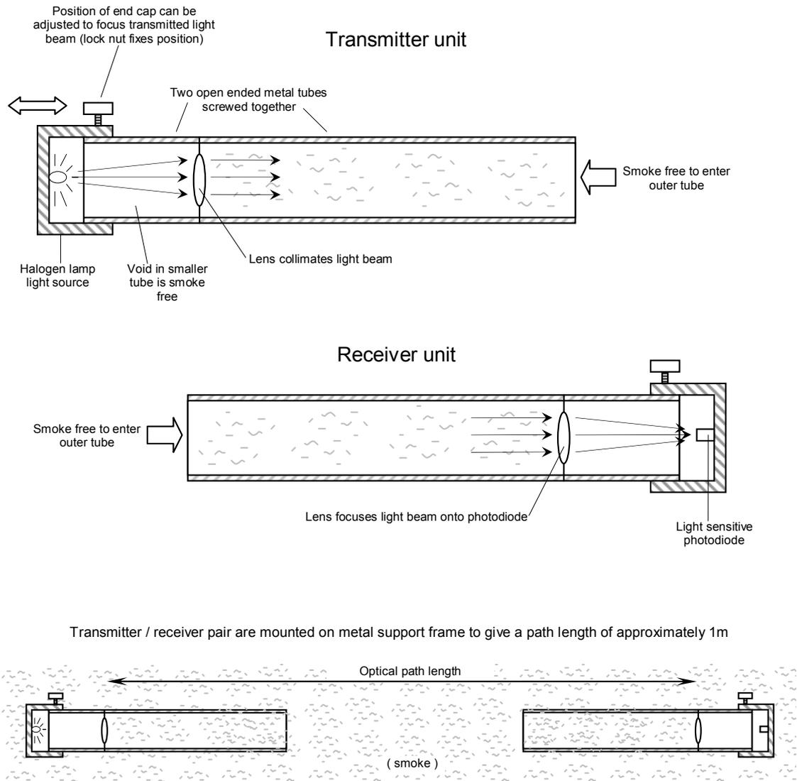
**Figure 5.6 Schematic of optical density meter**
