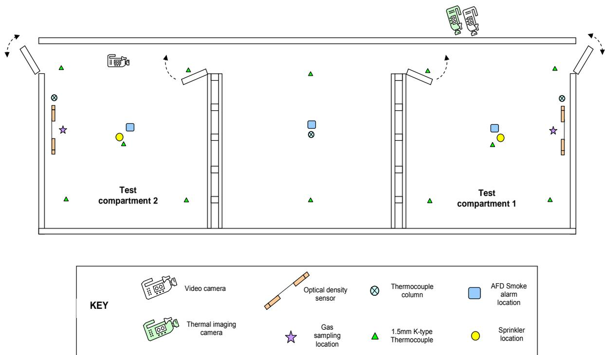
Figure 5.9 Schematic diagram showing the video and instrument locations
