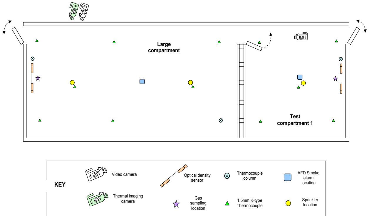
Figure 5.21 Schematic diagram showing the large compartment layout
