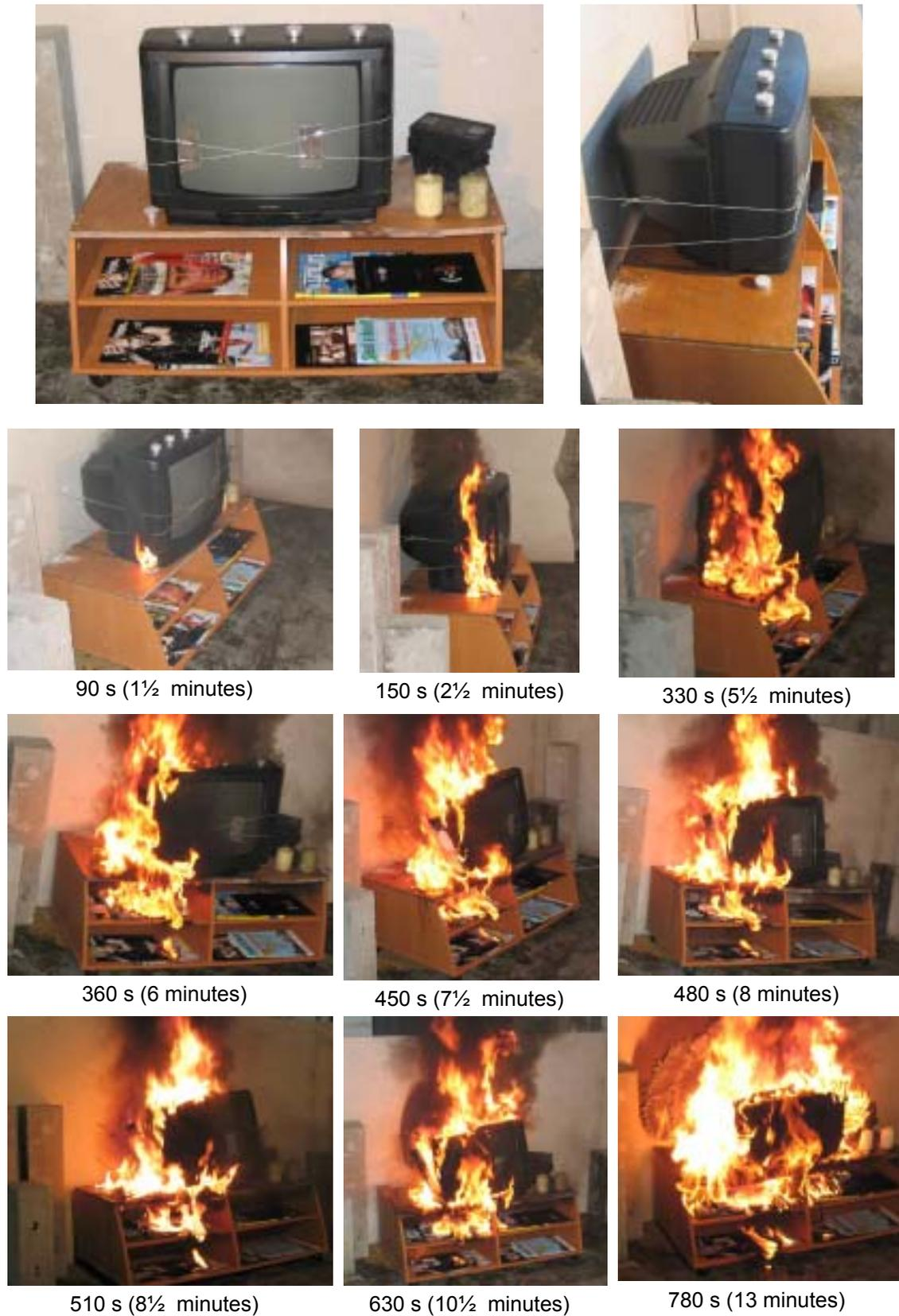
**Figure 5.27** Photographs taken before and during television calorimetry fire
