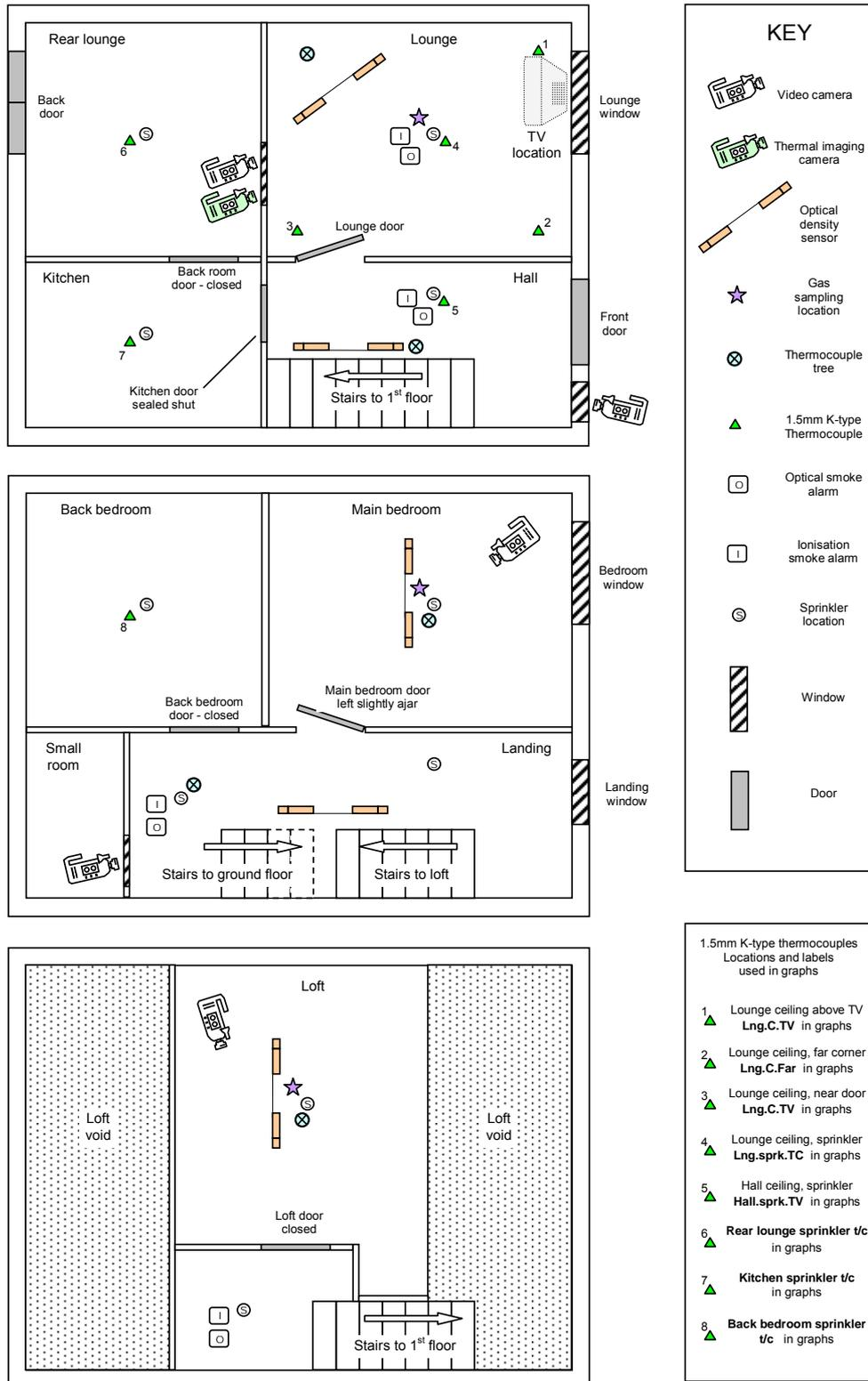
**Figure 5.2 Schematic diagram showing the internal layout of the house and instrument locations**
