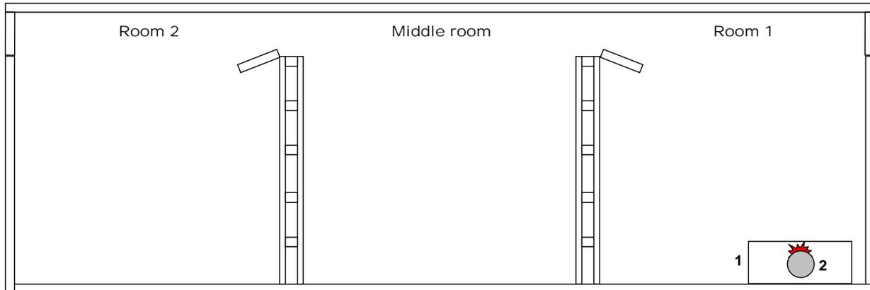
1-raised platform 2-oil pan
