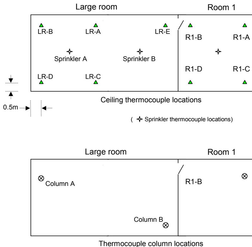
Figure 5.22 Thermocouple locations and nomenclature (for graphs)
