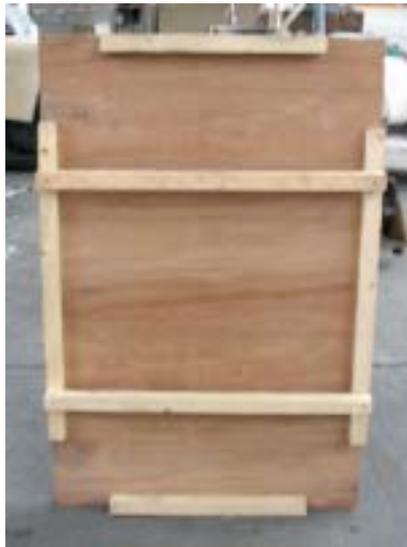
Plywood table top with wooden battens
