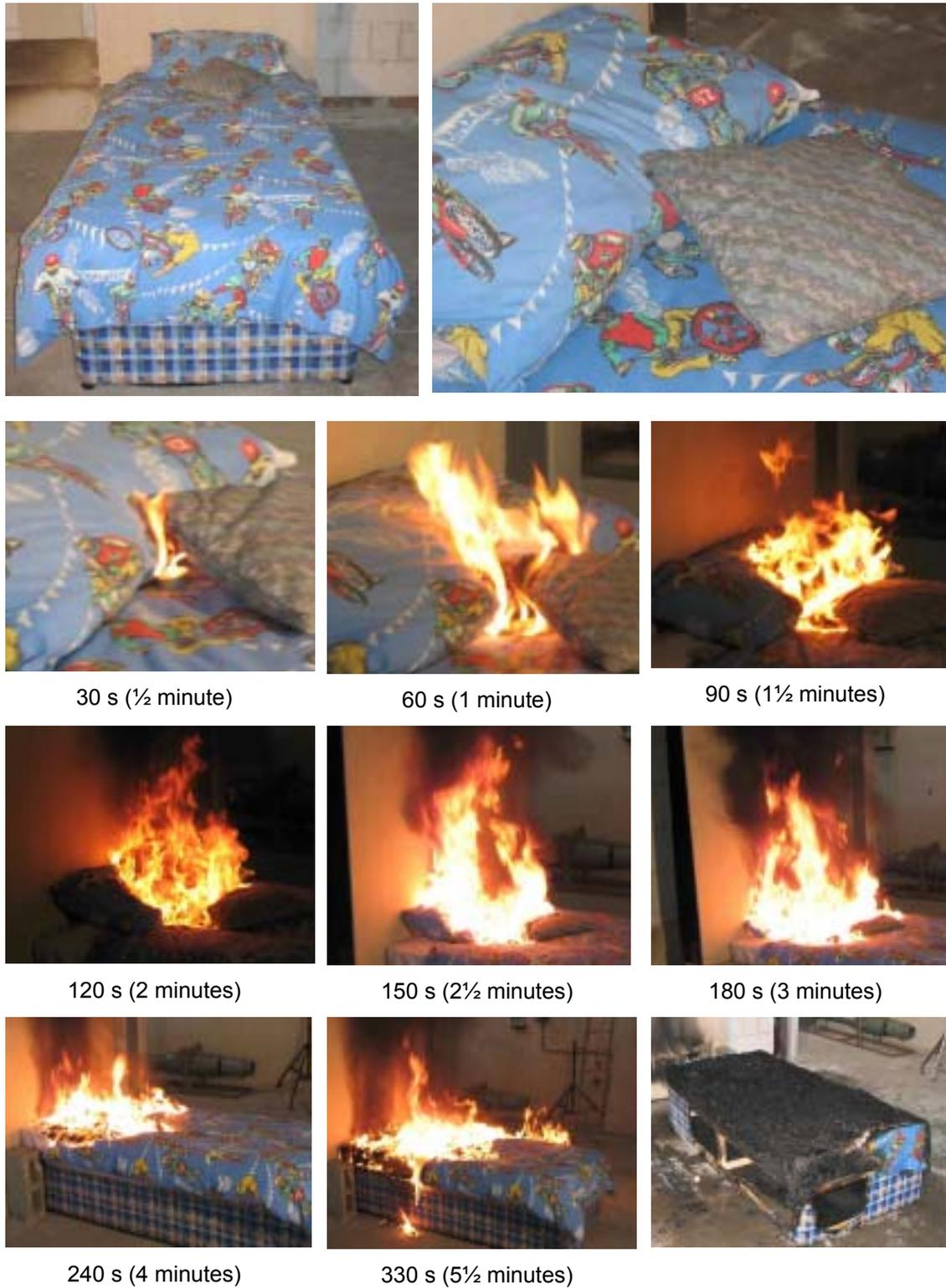
**Figure 5.30** Photographs taken before, during and after bed calorimetry fire
