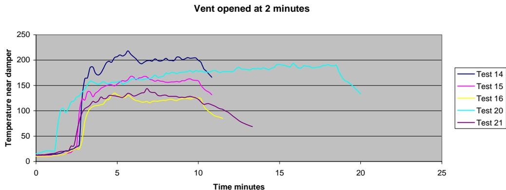
**Figure 11. Temperatures near the damper with the vent open at 2 minutes.**
