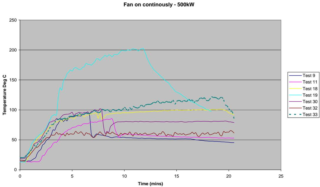
Figure 8. Temperatures near damper for the fan on and 500kW fire exposure.
