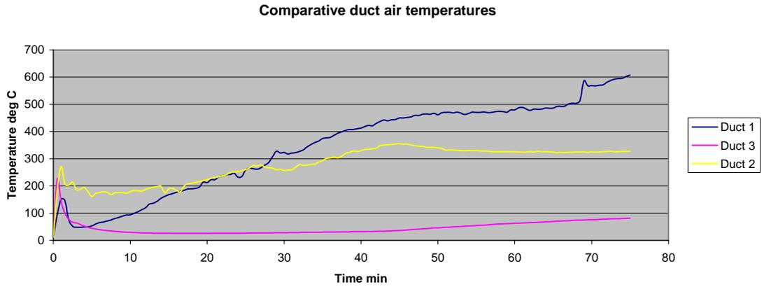
**Figure 12. Temperatures 500mm from damper during test**
