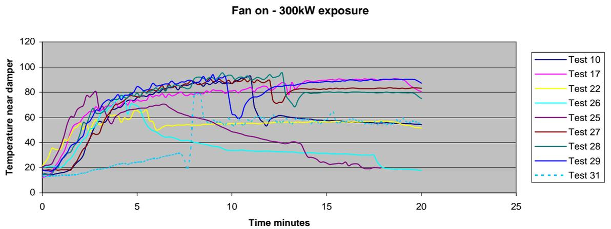
**Figure 9. Temperatures near damper for the fan on and 300kW fire exposure.**
