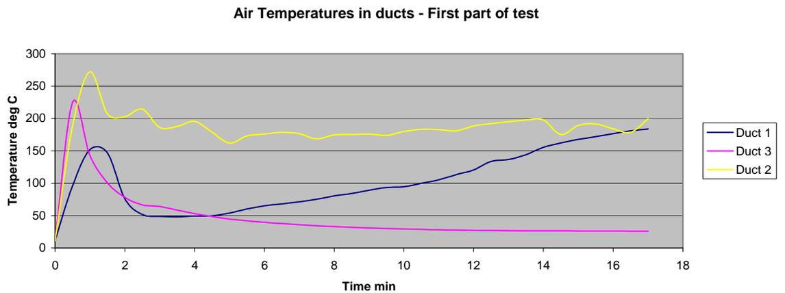
**Figure 13. Temperatures 500mm from damper in first 17 minutes of test**
