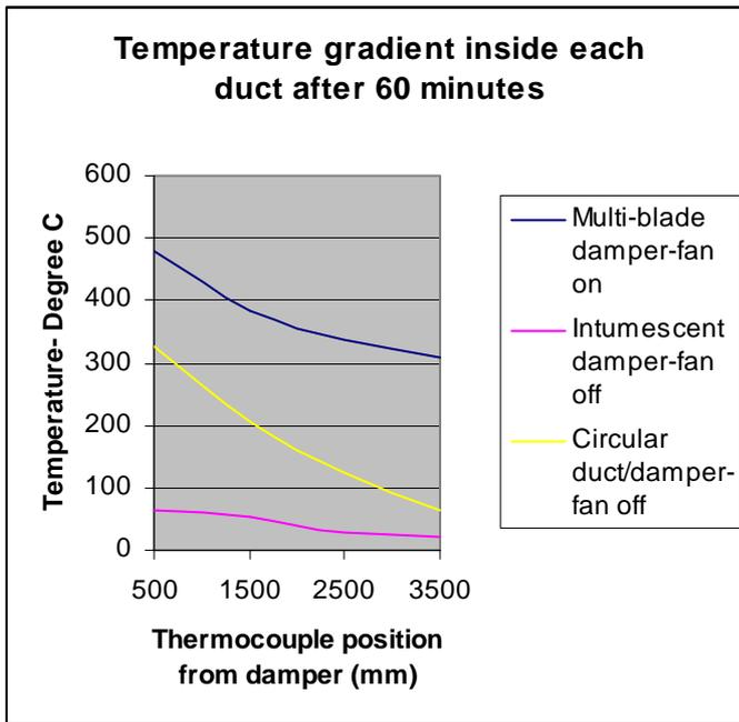
**Figure 15. Temperature gradient inside each duct at 60 minutes**
