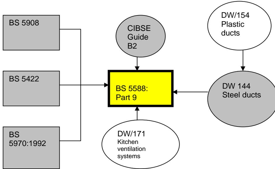
**Figure 3. Basic Code framework for HVAC systems**
