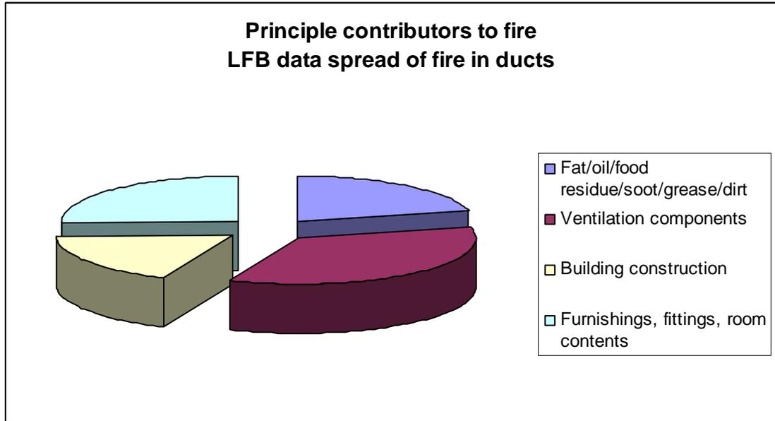
**Figure 7. Principle causes of fire spread in ducts**
