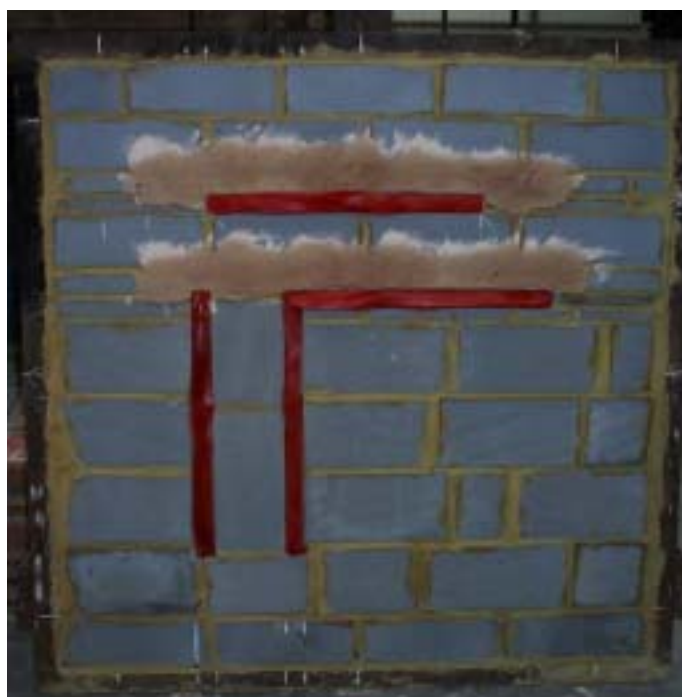
Photograph E6. Material installed in test frame
