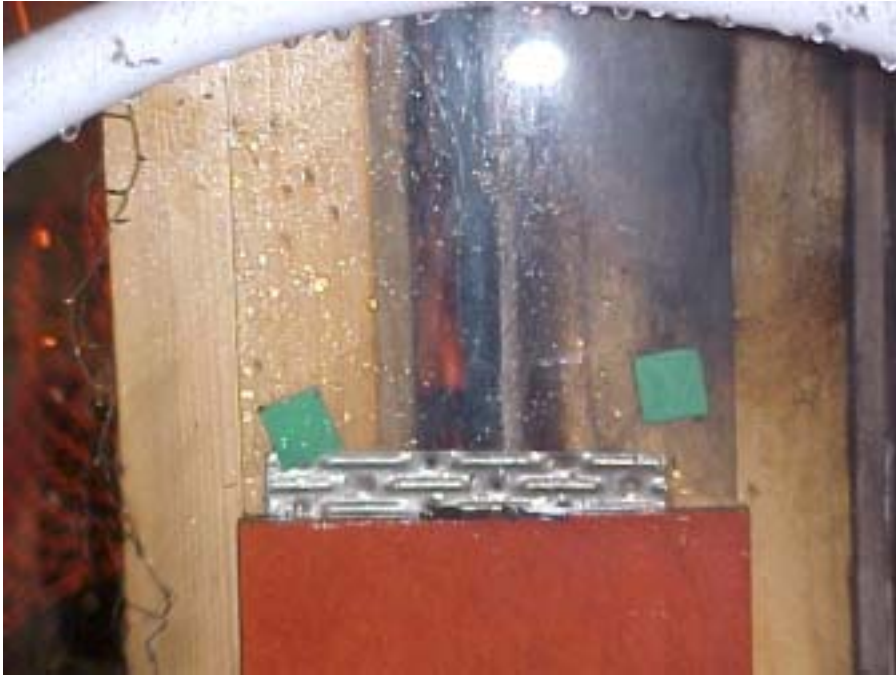
Photograph C4. Showing flaming entering the cavity.
