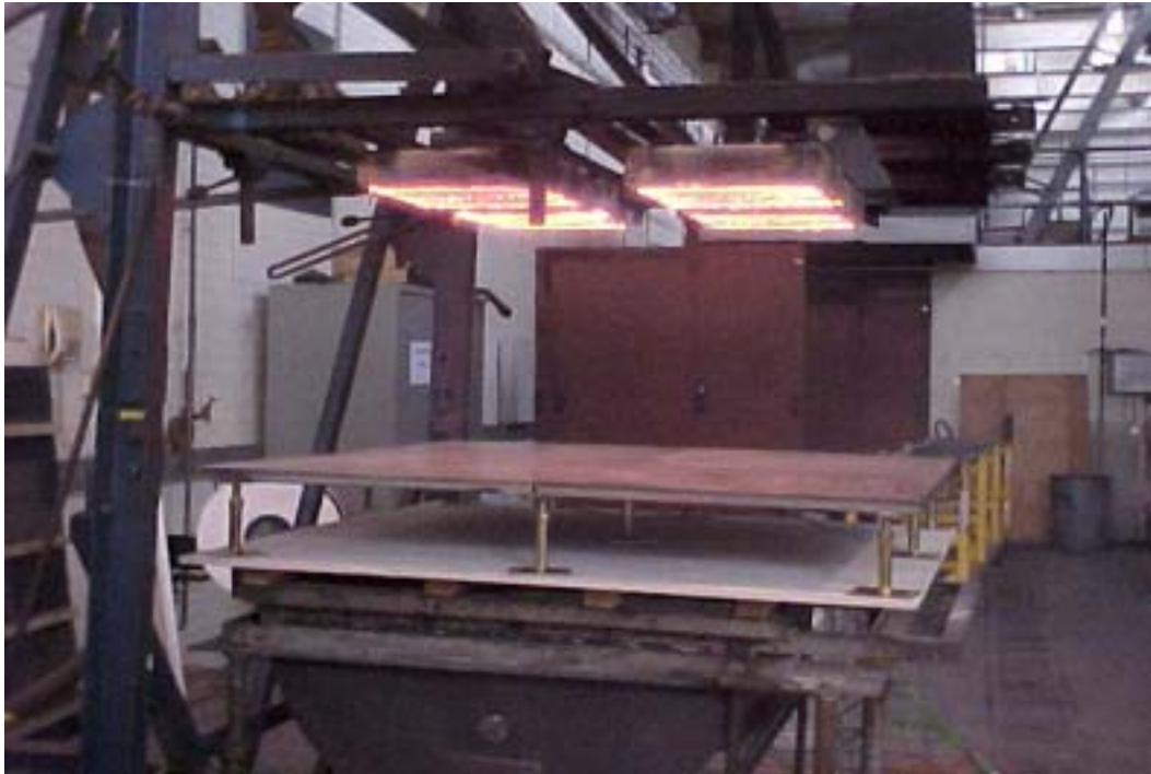
Photograph A19. Shows setup of test on radiant panel.
