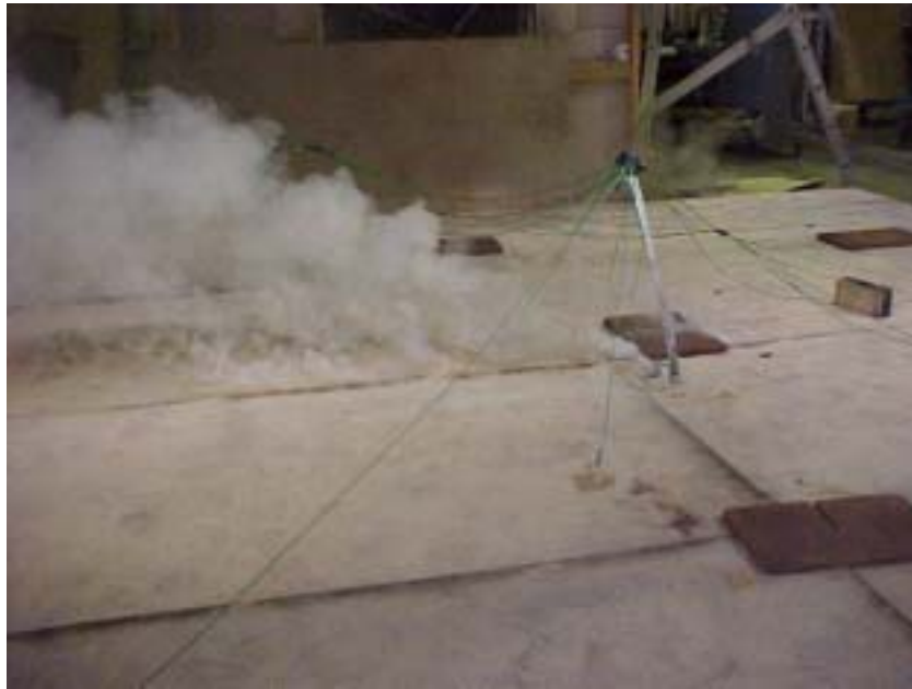
Photograph A17. Smoking from the chipboard floor.
