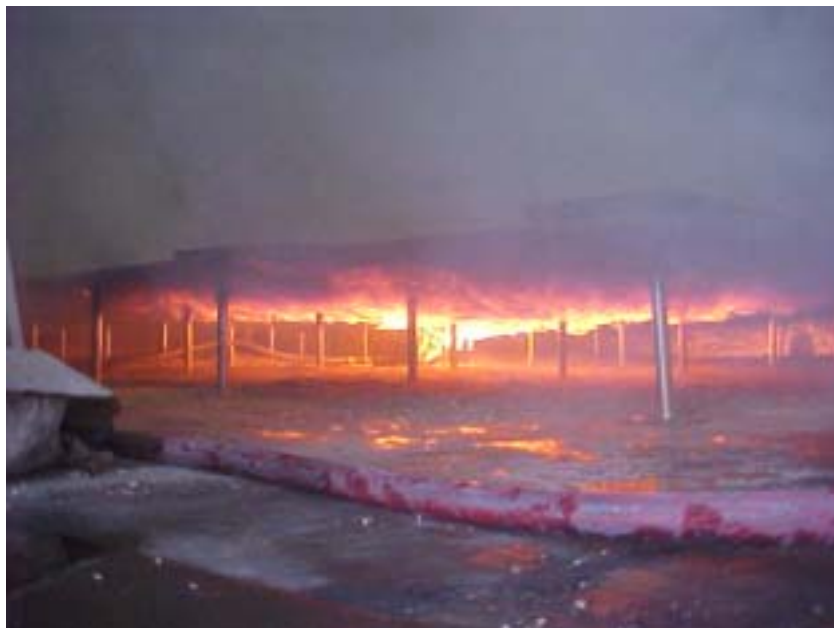
Photograph A18. Shows flames emerging from the edge of the floor.
