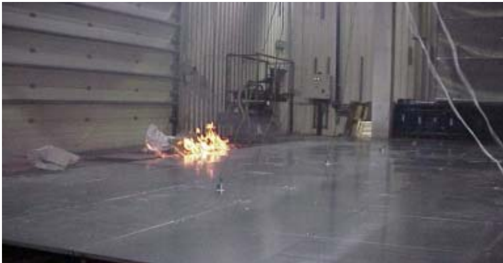
Photograph 12. flames emerging from the edge of the floor.
