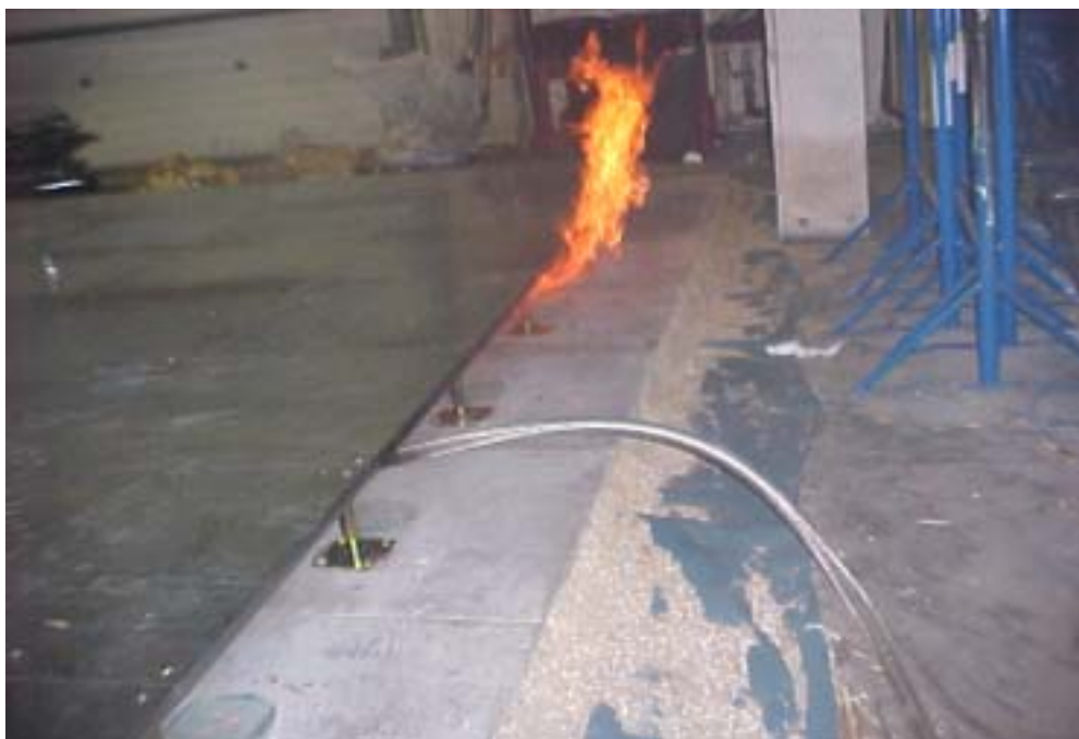
Photograph A15. Shows flames emerging from the edge of the floor.
