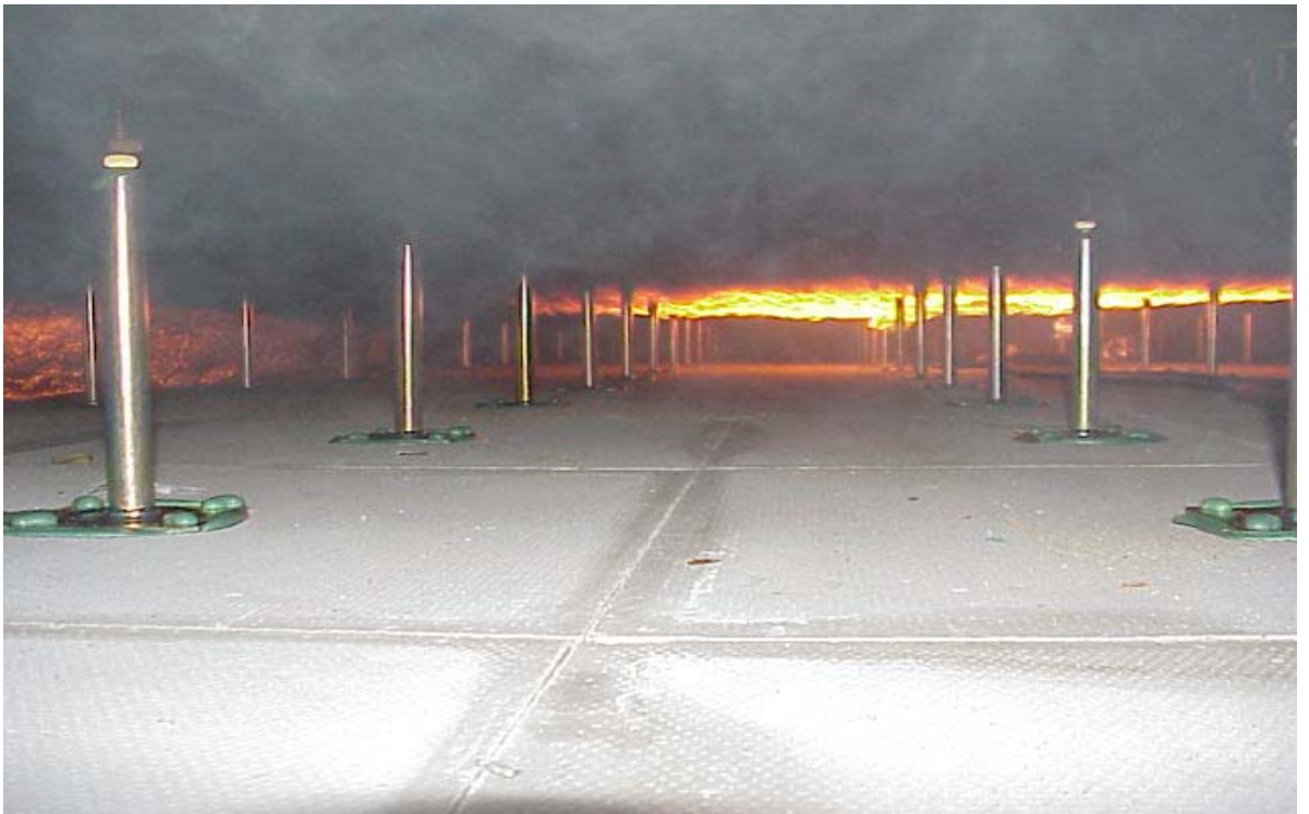
Photograph A6. Shows the flame spread under the floor, the cavity barrier can be seen on the left.
