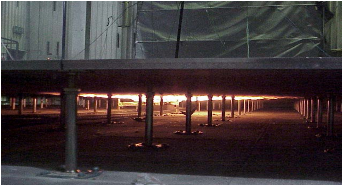
Photograph A9. Shows the flames spread away from the burner.
