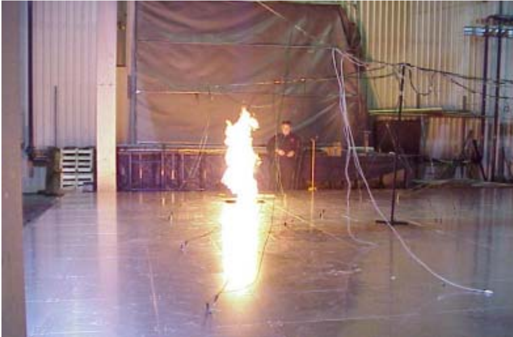
Photograph A5. Shows the burner being ignited, before being pushed under the floor.
