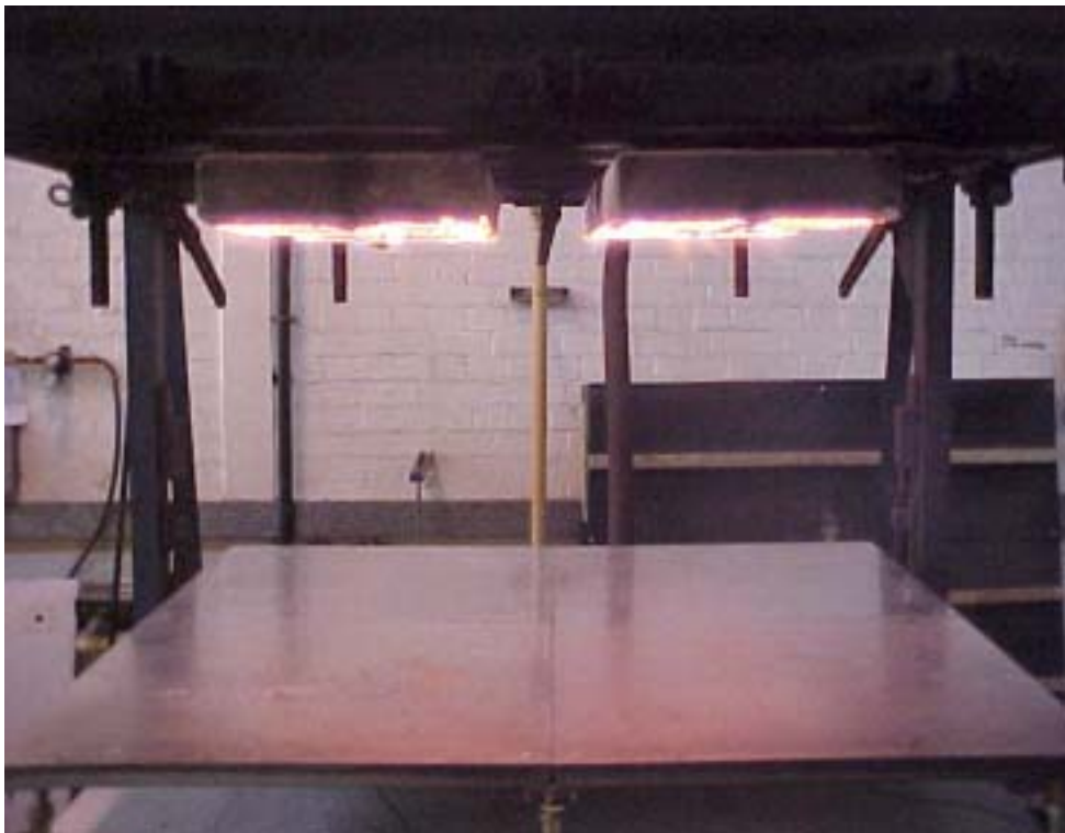
Photograph A20. Shows upper surface of floor being exposed to radiant heating.
