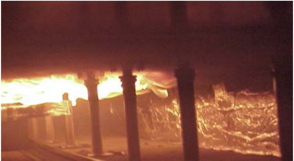
Photograph A7. Shows flames impinging onto the cavity barrier.
