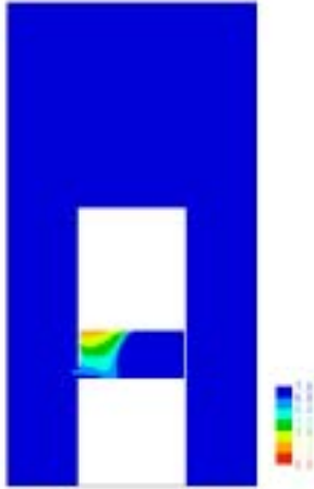
Lobby: L: 0.5m 2 low-level vent R: No vent Mean temp in occupied space = 28°C Closed door \Delta P = 90\text{Pa} ; open door vel = 1.6 ms -1
