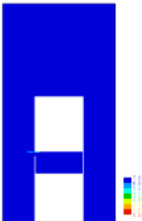
Lobby: L: 0.5m 2 high-level vent R: No vent Mean temp in occupied space = 22°C Closed door \Delta P = 90 \text{ Pa} ; open door vel = 1.4 ms -1
