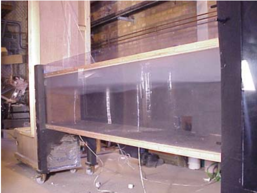
Figure B10 Photograph showing physical modelling Scenario 1 set with smoke layer in corridor entering large shaft
