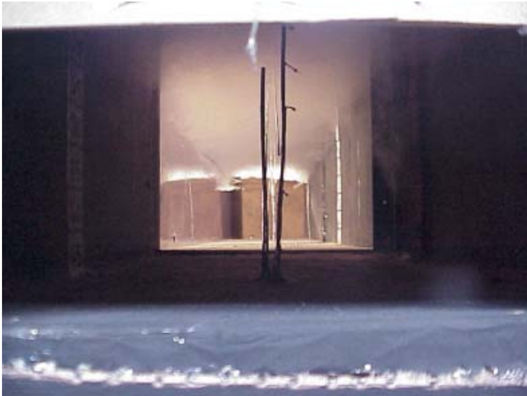
Figure B9 Smoke flowing along corridor from fire compartment
