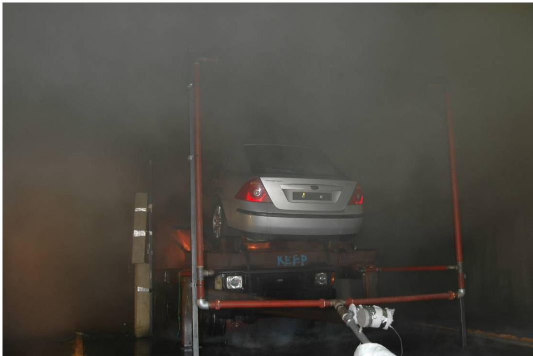
Figure 28 – BAFSA test in progress; 20 minutes 53 seconds after ignition
