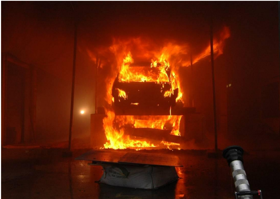
Figure 27 – CLG test in progress; 20min 59secs from ignition
