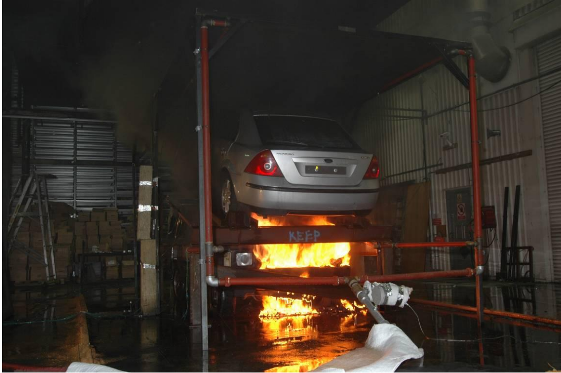
Figure 12 – Test in progress; 1 hour 23 minutes 9 seconds from ignition (sprinkler system off)
