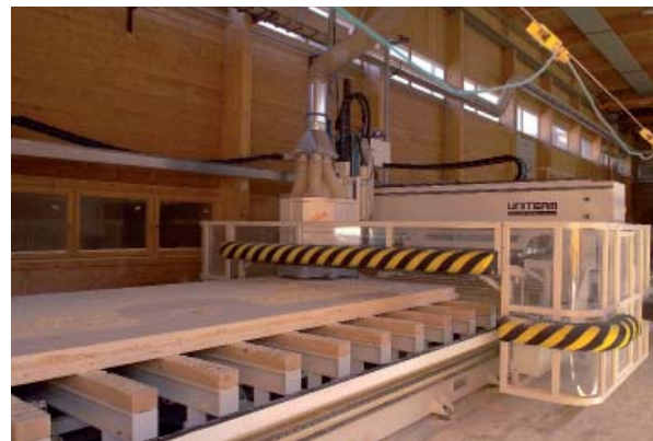
Figure 3: Manufacture of CLT (Courtesy of KLH)
