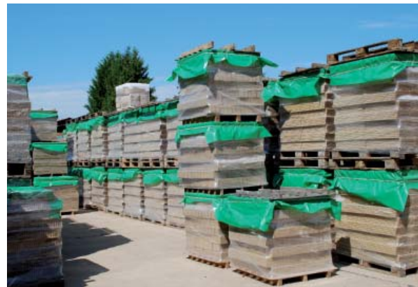
Figure 4: Careful storage of unfired clay bricks is important (Courtesy of University of Bath)
