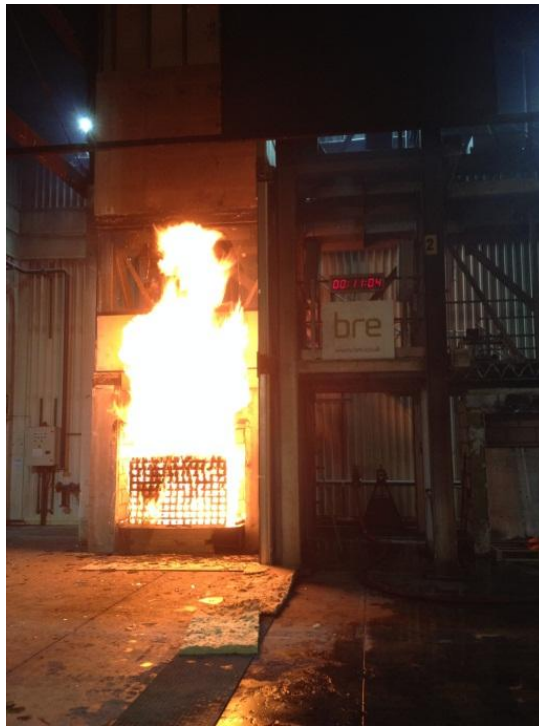
Figure 4 – Image showing maximum achieved flame length of approximately 3.3 m
