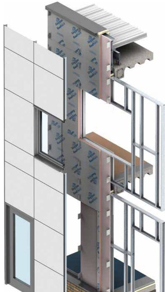
Figure 1 Architectural façade panel system; Kingspan
