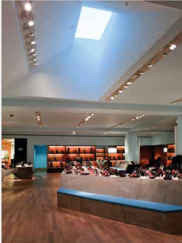
Figure 26: The shoes gallery at Selfridges: enhancement of space appearance and internal architecture by a combination of rooflights with dimmable electric lighting (© NDYLIGHT Lighting Designers and Consultants)
