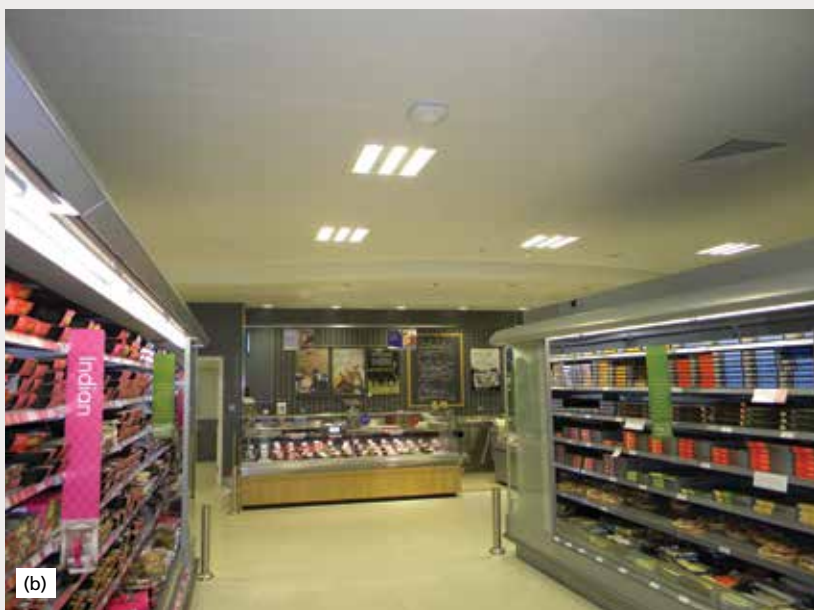
Figure 37: (a) John Lewis at Home (b) Waitrose. LED light sources used for accent and display lighting in shelves and display cabinets
