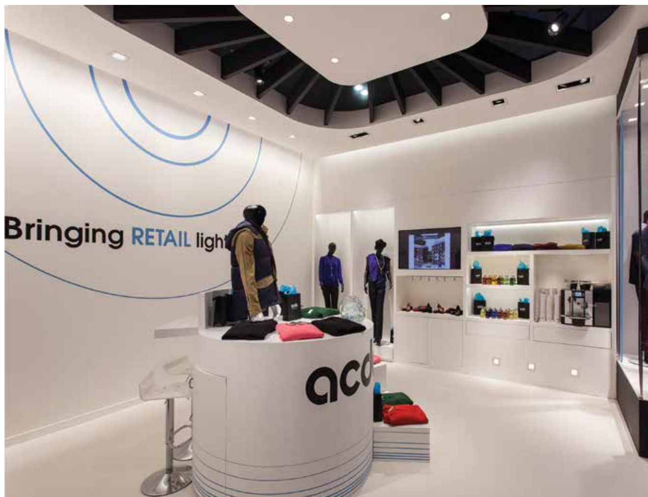
Figure 10: Perimeter lighting improving space appearance and size (© acdc)
