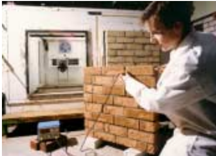
Testing masonry for frost resistance
