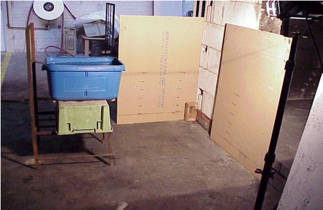
Figure 3 Photograph of splash test rig
