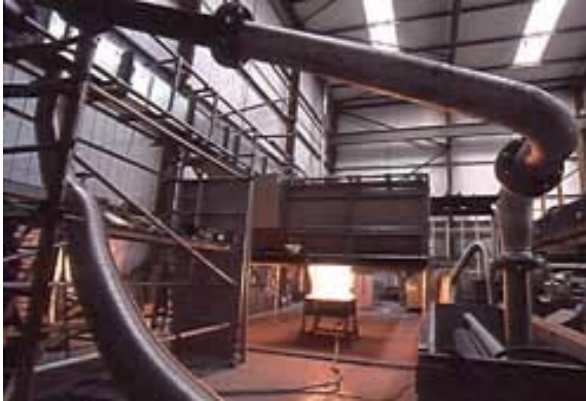
Plate 2. Photograph of a test to determine the activation time of a damper showing the fire source under the ceiling area with downstand.
