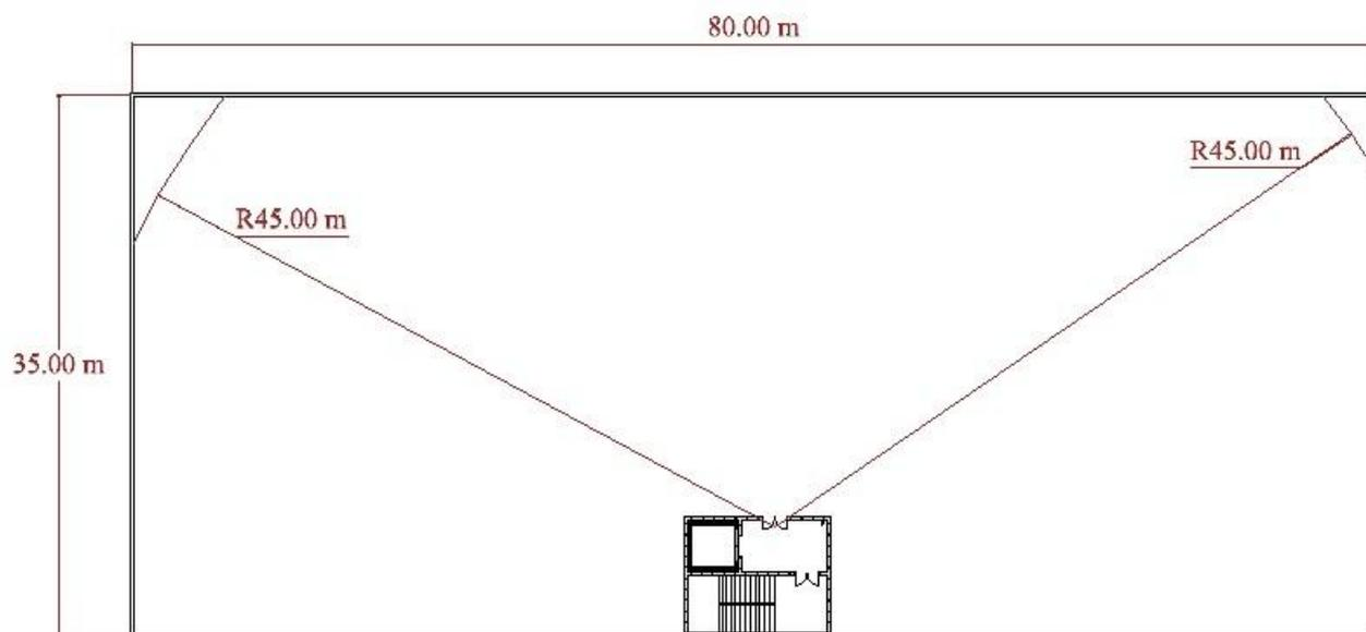
**Figure 5** Rectangle 2 – Note that a single shaft would not be adequate. An additional rising main will be necessary.
