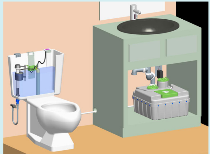
Figure 6 Greywater recycling system ( www.watersavetech.com )
