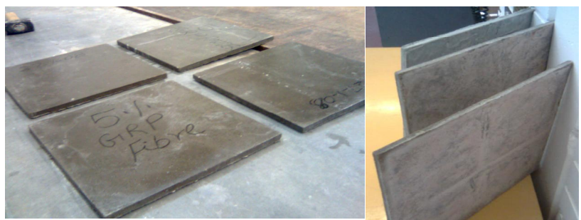
Figure 6: Architectural cladding panels from GRP waste fibre
