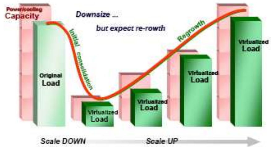
Fig 4b – Right-sized power/cooling Scaled capacity maximizes efficiency
