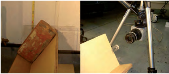
Figure 4: Laboratory experimentation to explore the behaviour of rain drops on masonry
