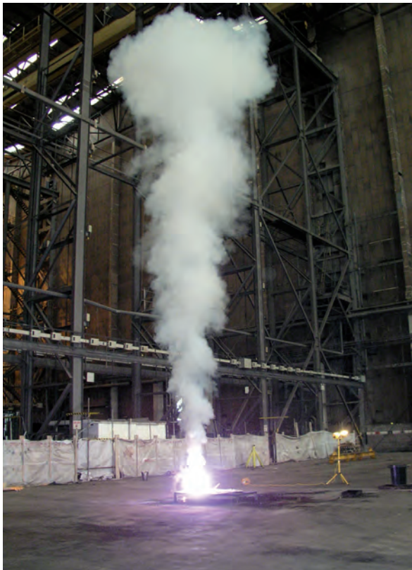
Figure 2: Smoke plume from a potassium lactose test fire in a 43.5 m high hangar
