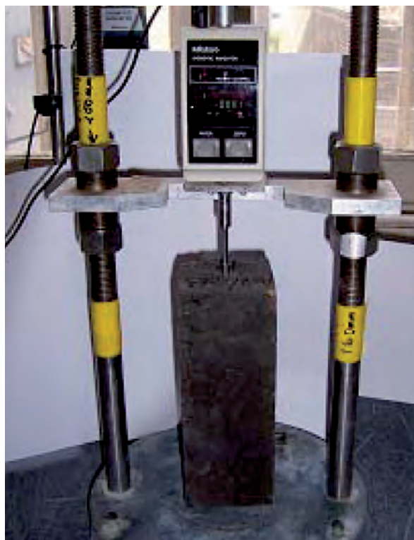
Figure 3: Expansion measurement for the ASR test
