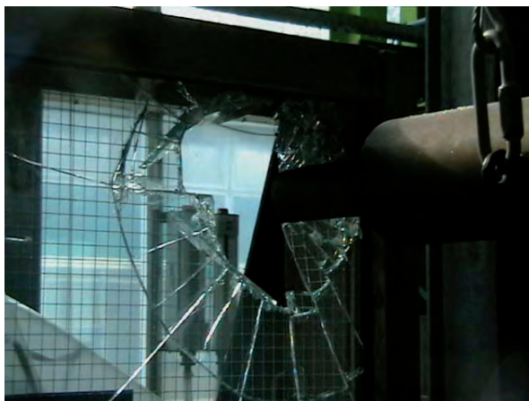
Figure 4: Hole formed in top corner of wired glass sample as a result of the first hard body impact
