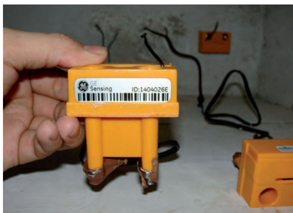
Figure 3: Setting up the hygrothermal monitoring of a thick stone wall in North Wales
