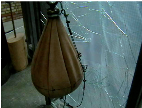
Figure 2: Leather spheroconical bag used to conduct soft body impact tests
