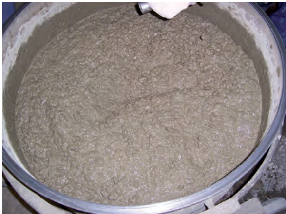
Figure 4: Alkali-activated concrete mix
