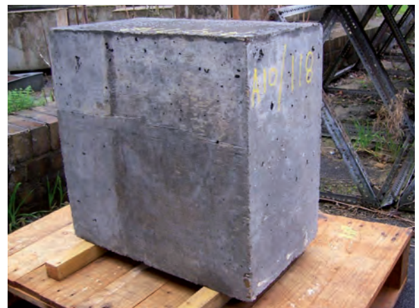
Figure 1: AAT wall block
