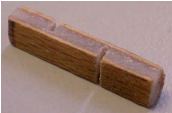
Figure 1: Miniature laminated veneer/adhesive/veneer specimen with offset cuts for creep in shear
