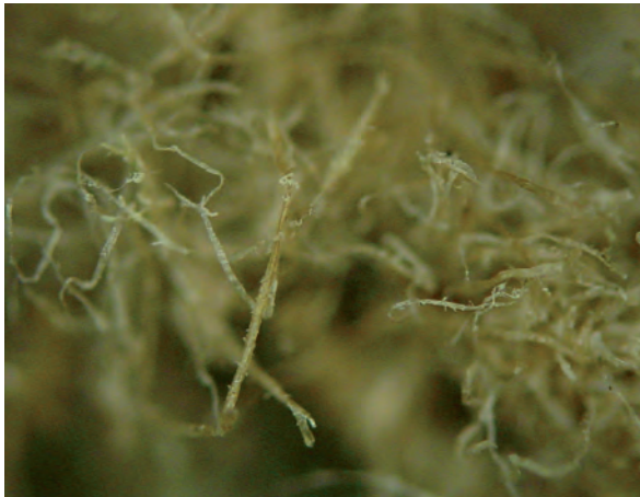
Figure 2: Sample of milled fibres produced from typical municipal black bag waste
