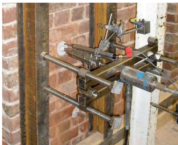
Figure 2: Pull-out test using a frictional device: set-up and instrumentation
