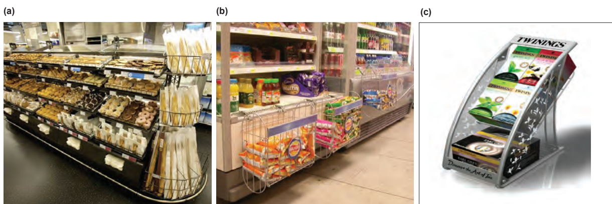
Figure 1: Examples of common shopfitting display equipment: (a) freestanding display that stands on its own and can be moved, (b) parasite display hanging from or attached to other displays, (c) shelf and counter display
