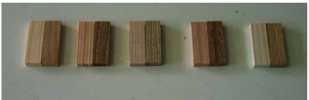
Figure 2: Enhanced coloration of timber with propolis treatment
