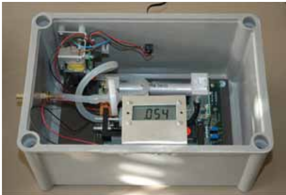
Figure 2: Butane sensor instrument developed by BRE
