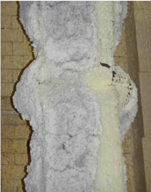
Figure 1: First loaded column. Note localised buckling of the steel in left-hand photo
