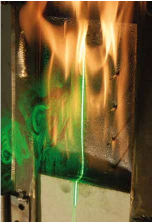
Figure 1: Final stages of an upward flame spread experiment
