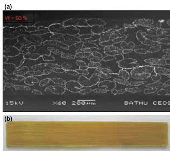
Figure 1: (a) Cross-section through sisal-PLA composite, (b) external appearance of composite
