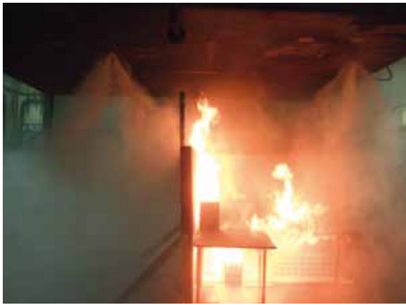
Figure 1: High-pressure water mist system in operation with BRE office fire test protocol
